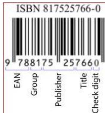
Verify that ISBN mentioned above with check digit is correct or not by using Modulo 11 system.
